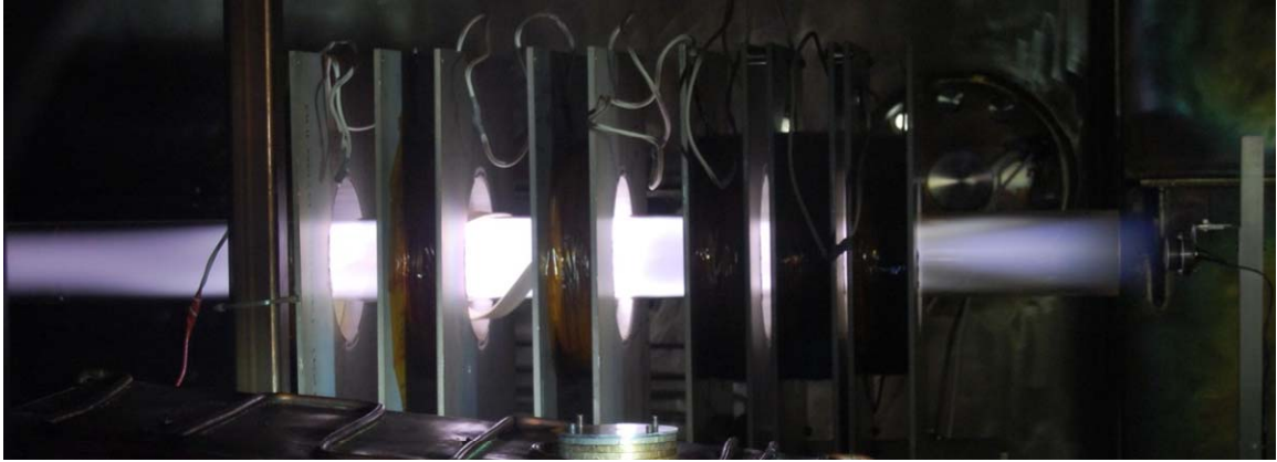
Figure 2.3: MadHeX thruster operating on argon while immersed in a vacuum environment at Georgia Institute of Technology.
