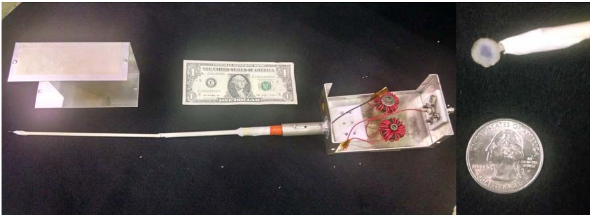
Figure 5.9: (Left) RF-compensated probe assembly with Langmuir probe tip attached and modified compensation circuit. (Right) Planar tungsten probe tip.
